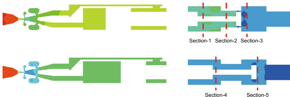
Fig. 6 Pressure monitoring surface of upstroke (upper) and pressure monitoring surface of downstroke (lower)
