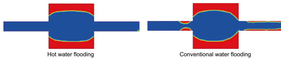
Fig. 18 Difference in residual oil and water distribution between conventional and hot water flooding after water broke through (Lv and Wang 2015)
