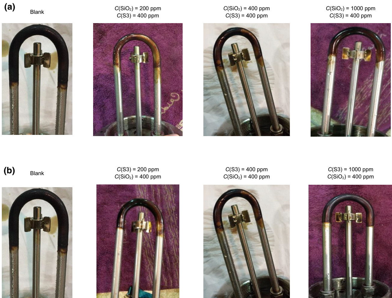
Fig. 6 Physical appearance of the deposited wax from treated crude oil at various concentrations. a Cold finger U-tube treated by SN3 with different concentrations of \text{SiO}_2 nanoparticles, b Cold finger U-tube treated by SN3 with different S3 concentrations
