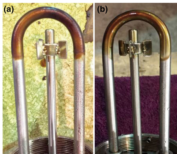
Fig. 13 Comparison between the physical appearances of the wax deposited on blank and treated samples at 18 °C. a Blank sample at 18 °C, b SN3-treated sample at 18 °C
