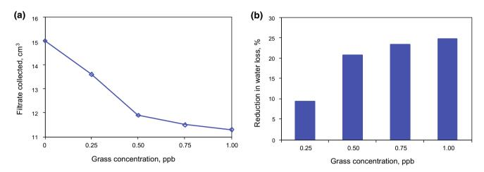
Fig. 5 Filtration characteristics of drilling fluids formulated with grass particles of 300  $\mu$ m
