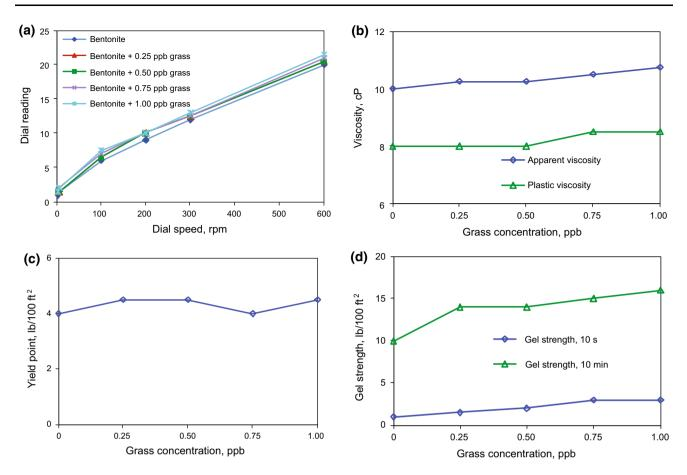
Fig. 7 Plot of rheological parameters for drilling fluids formulated with grass particles of 90 µm
