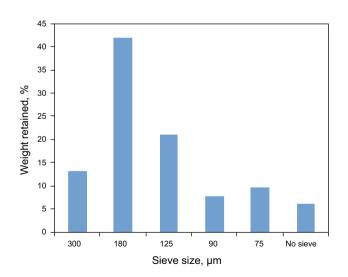
Fig. 1 Normal distribution curve of the grass sample on various sieves
