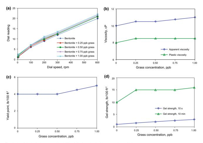
Fig. 4 Plot of rheological parameters for drilling fluids formulated with grass particles of 300 µm
