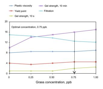
Fig. 12 Selecting the optimal concentration for 35-µm grass particles
