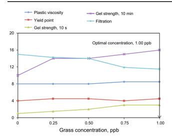
Fig. 9 Selecting the optimal concentration for 90-µm grass particles
