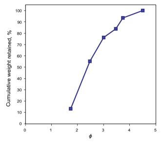
Fig. 2 Frequency distribution curve of the grass sample (where  $\phi$  is a dimensionless unit of the sieve sizes and is defined as  $\phi = -\log_{10}d/\log_{10}2$
