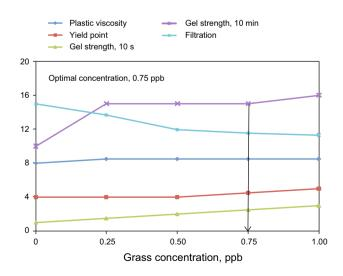
Fig. 6 Selecting the optimal concentration for 300-µm grass particles
