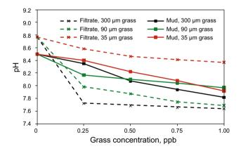
Fig. 13 Effect of the concentration of grass particles on pH of bentonite drilling fluids
