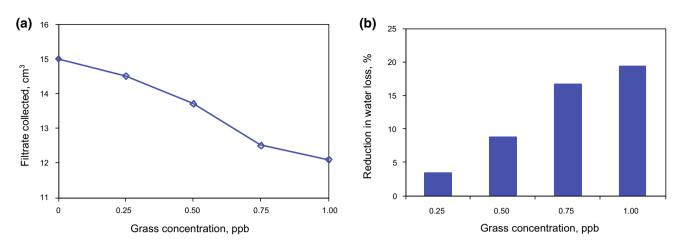
Fig. 11 Filtration characteristics of drilling fluids formulated with grass of 35  $\mu$ m
