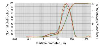
Fig. 3 Particle size distribution of the finest grass fraction obtained using a particle size analyzer
