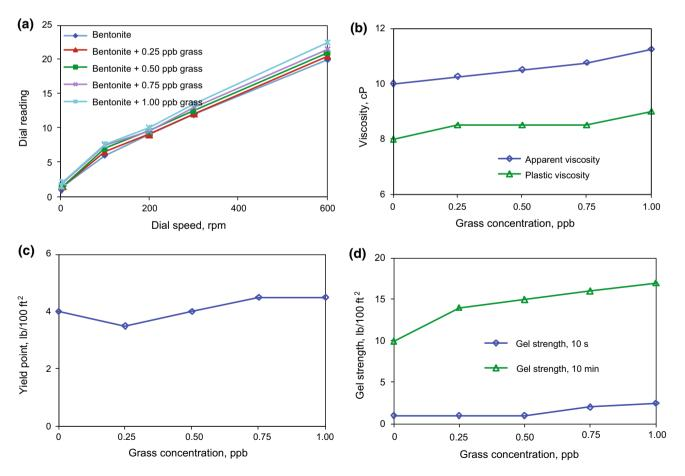
Fig. 10 Rheological parameters for drilling fluids formulated with grass particles of 35 µm
