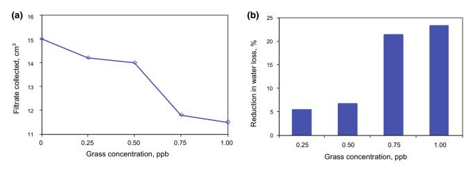
Fig. 8 Filtration characteristics of drilling fluids formulated with grass particles of 90  $\mu m$
