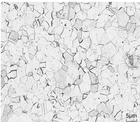
Fig. 4 Microphotograph of the inner pipe (316L)
