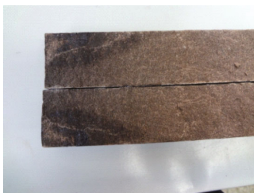
Fig. 6 Head face and profile of the core after direct injection of ethylenediamine
