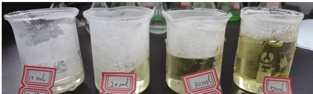
Fig. 3 Reaction products of ethylenediamine and CO 2 at 3 MPa
