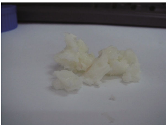
Fig. 5 The final product of the yellowish-brown viscous liquid continually exposed to CO 2
