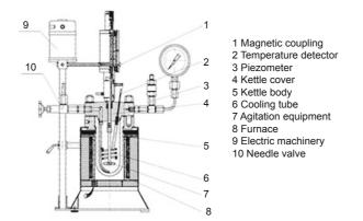
Fig. 1 Experimental device for emulsion polymerization—GSH reactor
