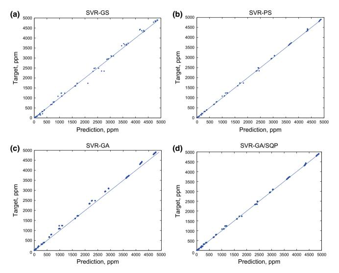
Fig. 5 The parity plot for different algorithms. a Hyper-parameter optimization using GS. b Hyper-parameter optimization using PS. c Hyper-parameter optimization using GA-d Hyper-parameter optimization using GA-SQP
