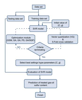
Fig. 3 The procedure of parameter tuning in SVR
