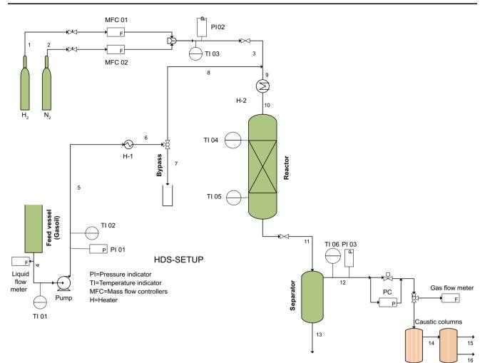
Fig. 2 Schematic of HDS set-up
