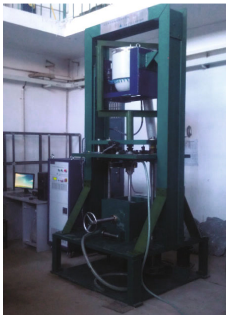
Fig. 3 The experimental vibration excitation apparatus
