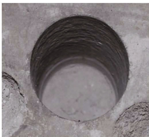
Fig. 12 The rock sample cut by a 100-mm-diameter PDC bit (sample 7#)
