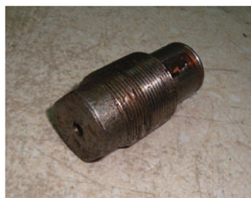
Fig. 6 A nozzle with 3 tangential inlets for swirling jet
