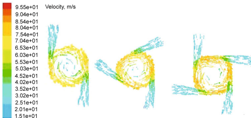
Fig. 3 Comparison of swirling flow near the tangential inlets
