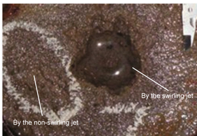
Fig. 9 Comparison of rock breaking at the same nozzle pressure drop
