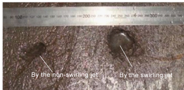
Fig. 8 Comparison of cavities created in the same rock sample at the same discharge
