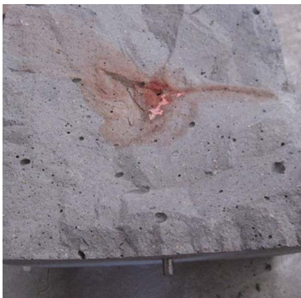
Fig. 7 Fracture propagation in specimen 8#
