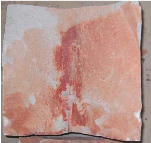
Fig. 5 Fracture propagation in specimen 3#
