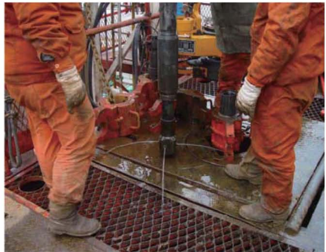
Fig. 9 Field test of rapid solution mining tool
