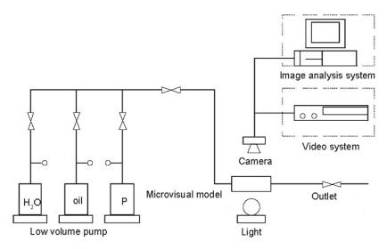
Fig. 3 The schematic diagram of microscopic oil displacement experiment
