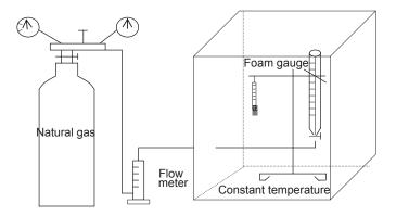
Fig. 1 A system for measuring the foaming properties of foaming solution
