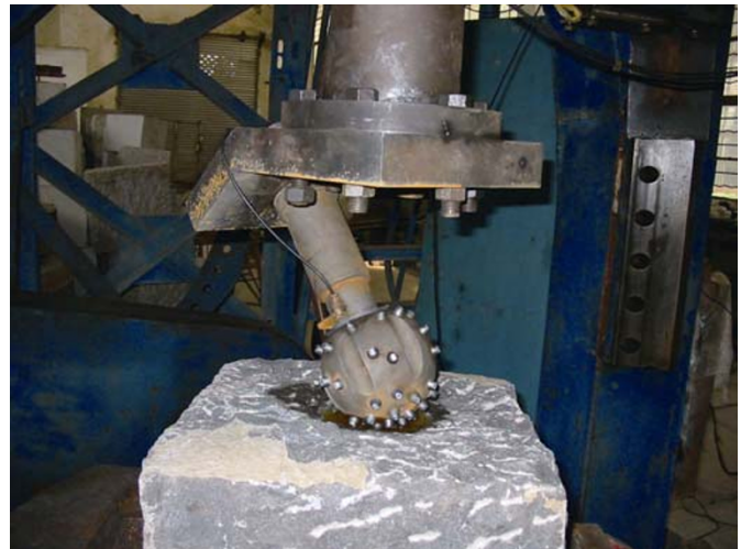
Fig. 2 Offset single-cone bit
