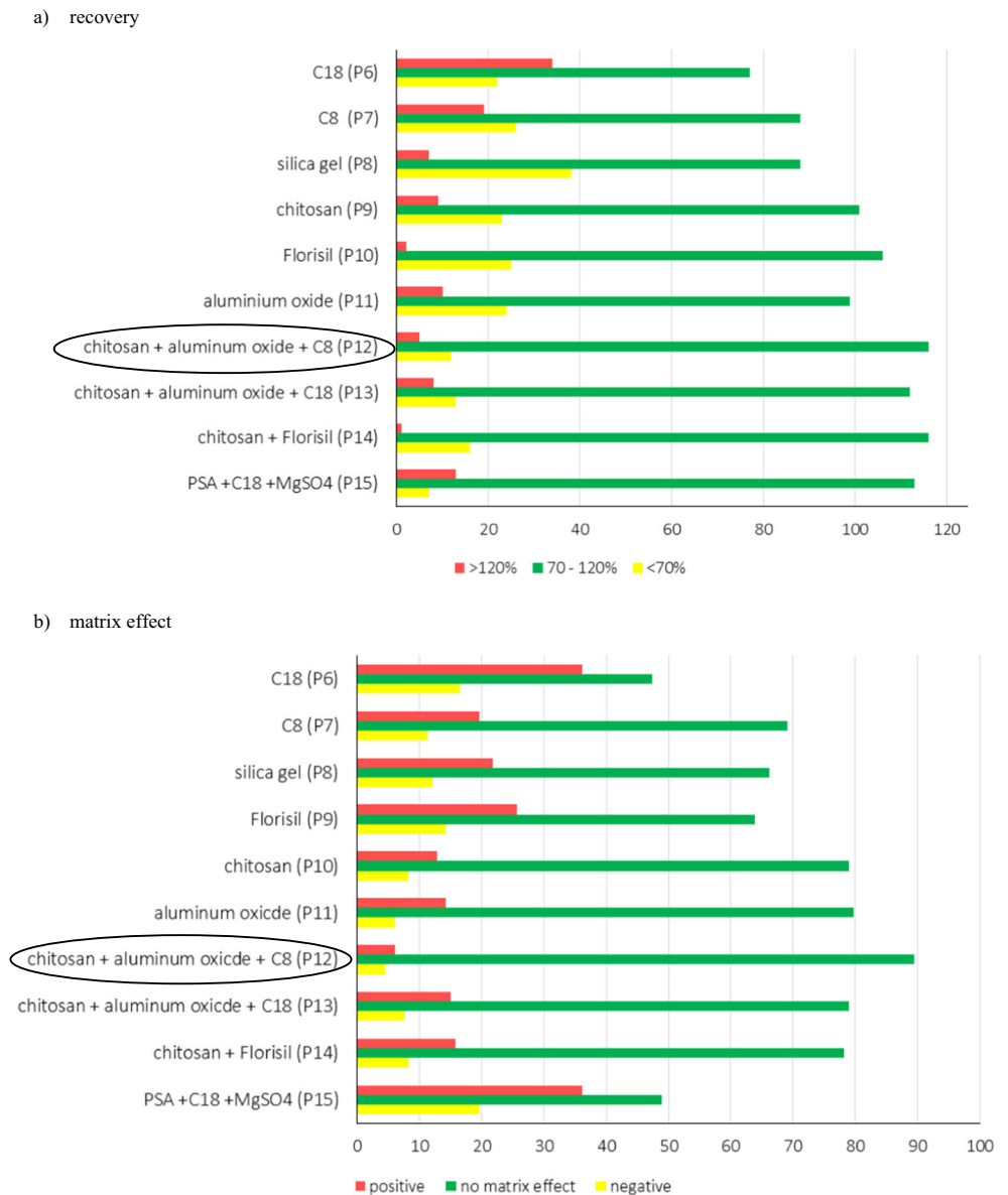
Fig. 3 Effect of different cleanup sorbents on recovery (a) and matrix effect (b) of 132 insecticides at 0.01 mg kg -1 (procedures P6–P15)
