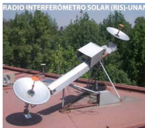
Fig. 1 The RIS consists of two antennas of 1 m of diameter in an equatorial mount and separated by 120 wavelengths
