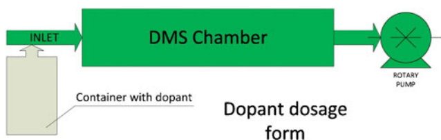
Fig. 7 Block diagram of “open” gas exchange system used in DMS chamber
