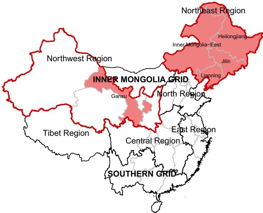
Fig. 1 Major grid regions (red borders) and provinces (red shading) of State Grid referenced in the market cases. All-caps labels refer to other grid companies
