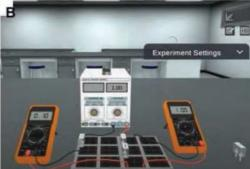
Figure 3. (A) Prepopulated lab bench to verify Ohm's law using Praxilabs. Students can opt for different connection types (single, series, and parallel) at the beginning of the experiment and choose the resistance value(s). (B) 'Zoomed-in' view of the experimental set-up. Students are provided with a power supply box, resistance box, and two multimeters. Students can measure the current using the ammeter and check the validity of Ohm's law based on other information.
