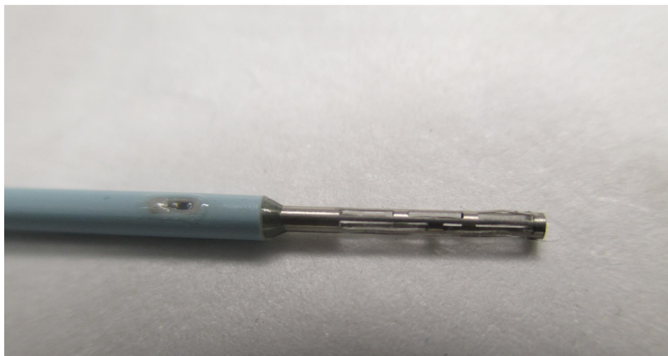
Fig. 3 Schematic illustration and photography of the MPBS. The computer-aided design drawing demonstrates the assembly of the different sensors as well as the dimension of the MPBS. The picture shows the tip of the MPBS with the ICP sensor on the left and distal steel cage on the right
