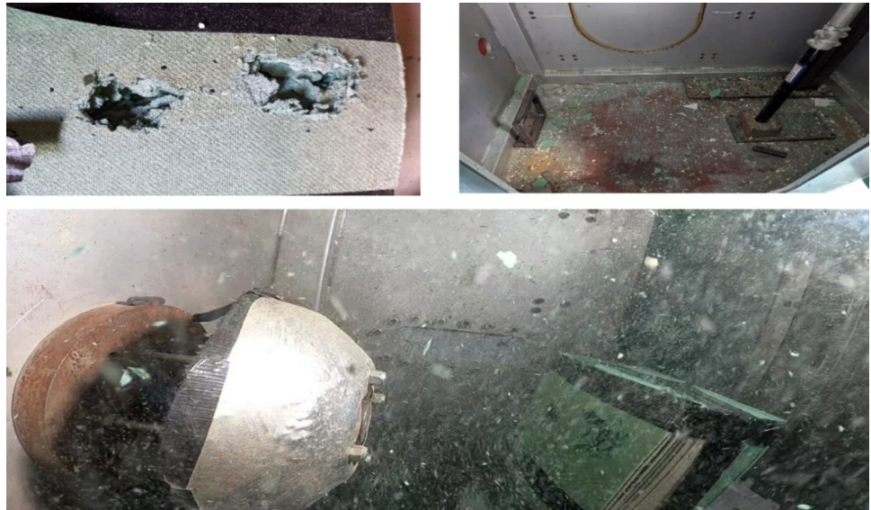
Fig. 8 Top Left: Underlay material sample post projectile impact. Top Right: Underlay debris within target chamber. Bottom Centre: Underlay Debris post projectile impact
