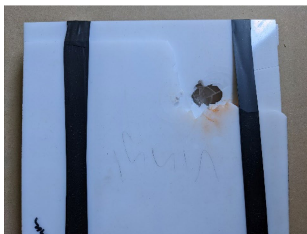
Fig. 7 PVC post impact damage
