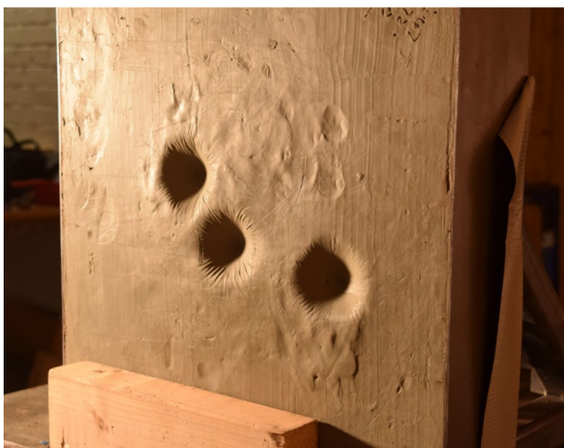
Fig. 6 Back face trauma from 67 ms -1 impact
