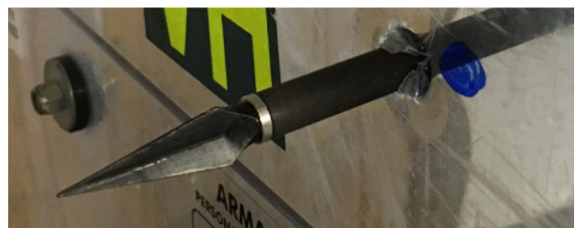
Fig. 10 Broadhead tip single skinned area perforation at 67 ms -1
