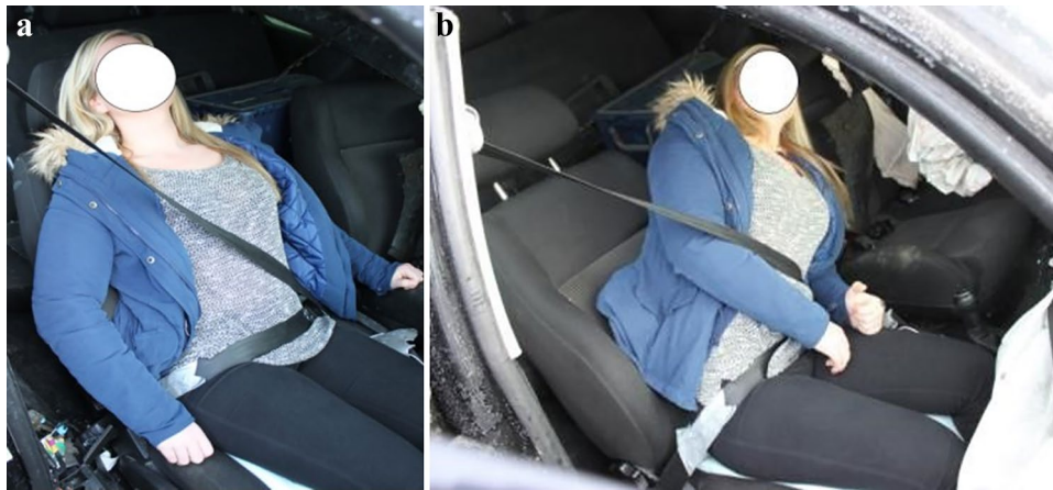
Fig. 5 Reconstruction of the injury mechanism for front-seat passenger involved in a collision. The main impact was to the left front of the MV. Seatbelt misuse due to improper occupant posture relative to seatbelt. The seatbelt did not tighten effectively across the occupant's torso during the collision (a). The shoulder part of the seatbelt was
