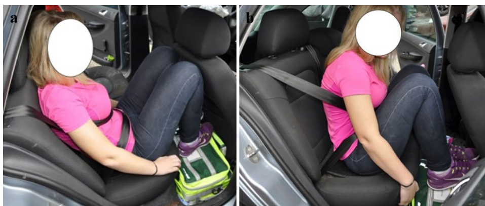
Fig. 6 Reconstruction of injury mechanism for right rear-seat passenger involved in a frontal collision. Seatbelt misuse due to incorrect routing of the seatbelt and improper occupant posture relative to the seatbelt. The shoulder part seatbelt was routed under the right arm and the lap belt was too high over the abdomen (a). Moreover, the occupant's legs were on top of luggage placed on the floor behind the
