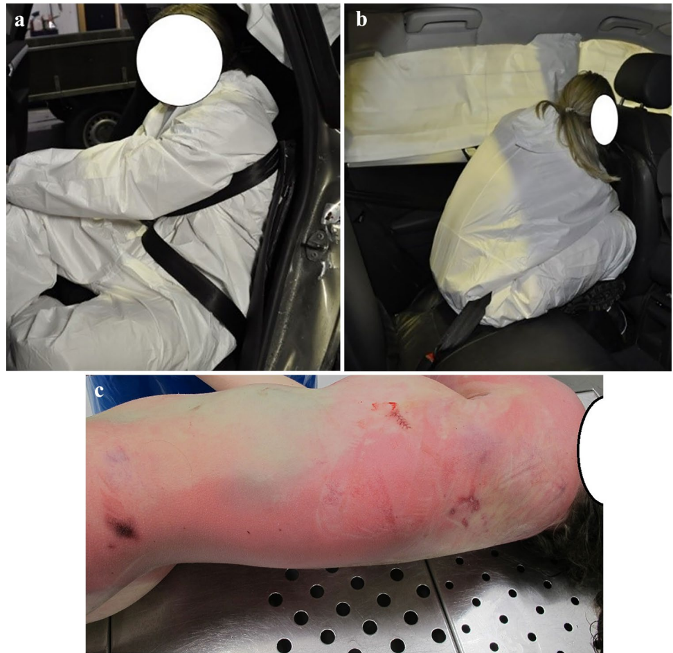
Fig. 7 Reconstruction of injury mechanism for left rear-seat passenger involved in a fatal nearside collision (a). Seatbelt misuse due to incorrect routing of the shoulder part of the seatbelt under the left arm that allowed for excessive forward movement of the head (b) and torso and direct contact with the driver's seat back. Insecure cargo in the trunk displaced the rear seatback >20 cm forwards, and increased the seatbelt loading on the torso. Injuries: Bruising and abrasion suggestive of seatbelt mark (c) was found under the left arm, as well as mandibular fracture, fatal traumatic brain injury, traumatic subarachnoid hemorrhage, C1-fracture, multiple rib fractures, and a major spleen rupture
