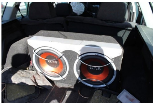
Fig. 9 Evidence of insecure heavy cargo in the trunk displacing the rear-seat row forwards in a frontal collision. Luckily, no occupants were sitting in the rear-seat row during the collision
