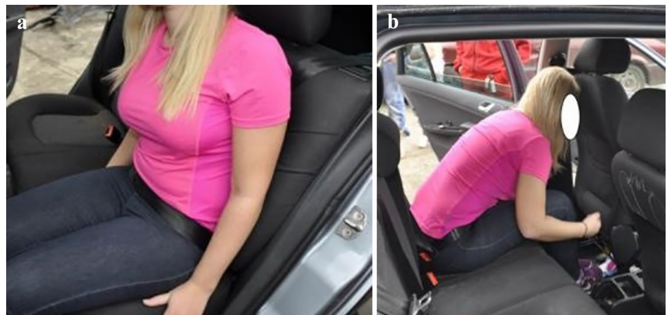
Fig. 8 Reconstruction of injury mechanism for left rear-seat passenger involved in a frontal collision. Seatbelt misuse due to incorrect routing of the seatbelt behind the back (a) allowing for excessive forward movement of the head and torso and direct contact with the driver seat back, displacing it >10 cm forward (b). Injuries: Luckily, only minor head contusion and lung contusions
