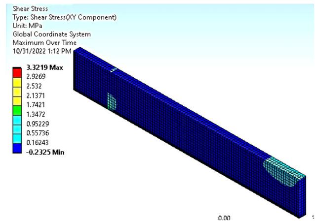
Fig. 11 FE contour of shear stress without crack
