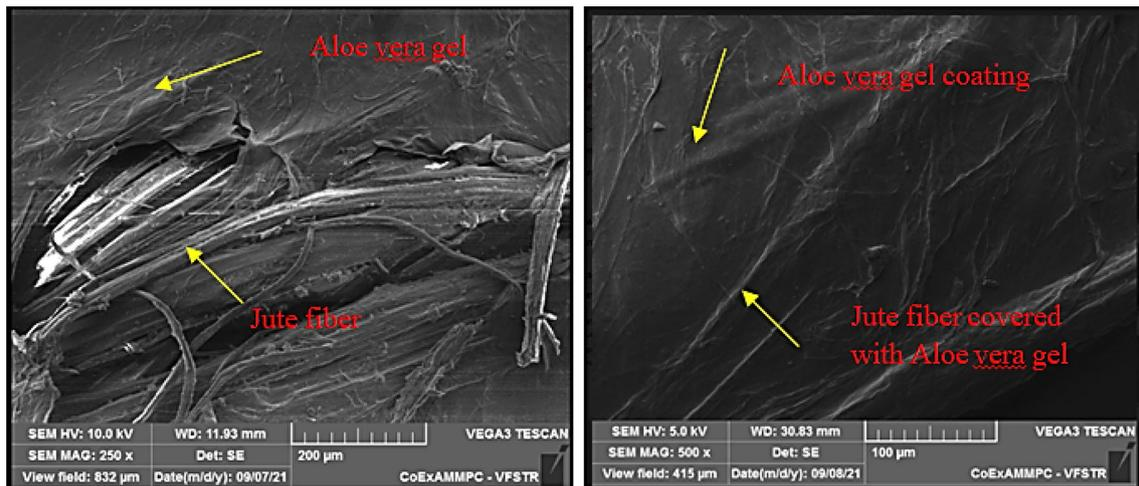
Fig. 6 SEM images of dried Jute fiber with aloe vera gel
