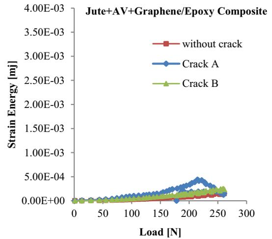
Fig. 25 Strain energy in Jute + AV + Graphene/E
