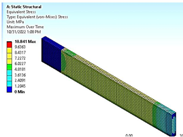
Fig. 10 FE contour of von Mises stresses without crack
