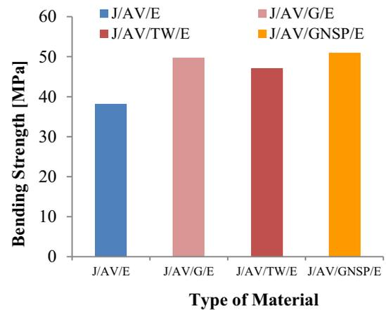
Fig. 4 Variation of bending strength
