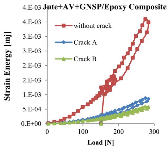
Fig. 17 Strain energy in Jute + AV + GNSP/E
