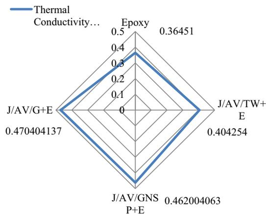
Fig. 7 Thermal conductivity of the natural composites
