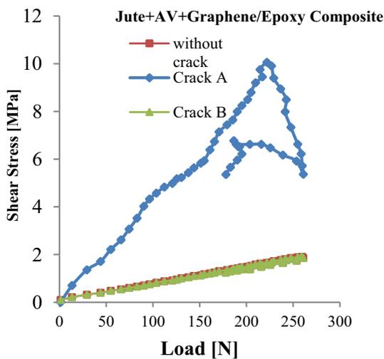
Fig. 23 Shear stress in Jute + AV + Graphene/E
