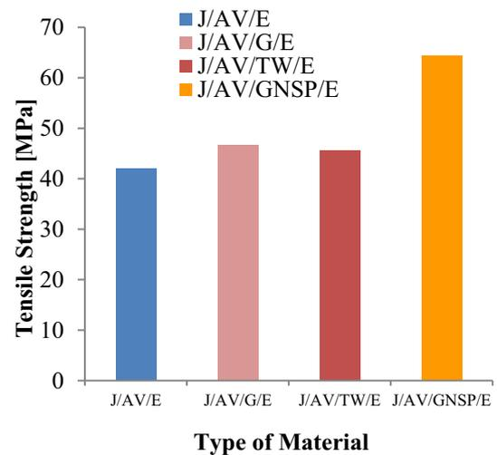
**Fig. 2** Variation of tensile strength
