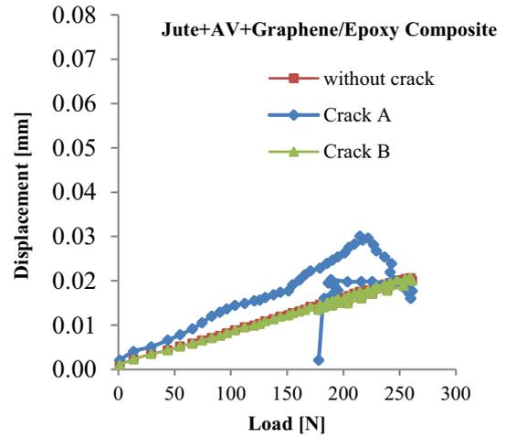
Fig. 24 Displacement in Jute + AV + Graphene/E
