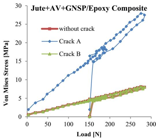
Fig. 14 Von mises stress in Jute + AV + GNSP/E
