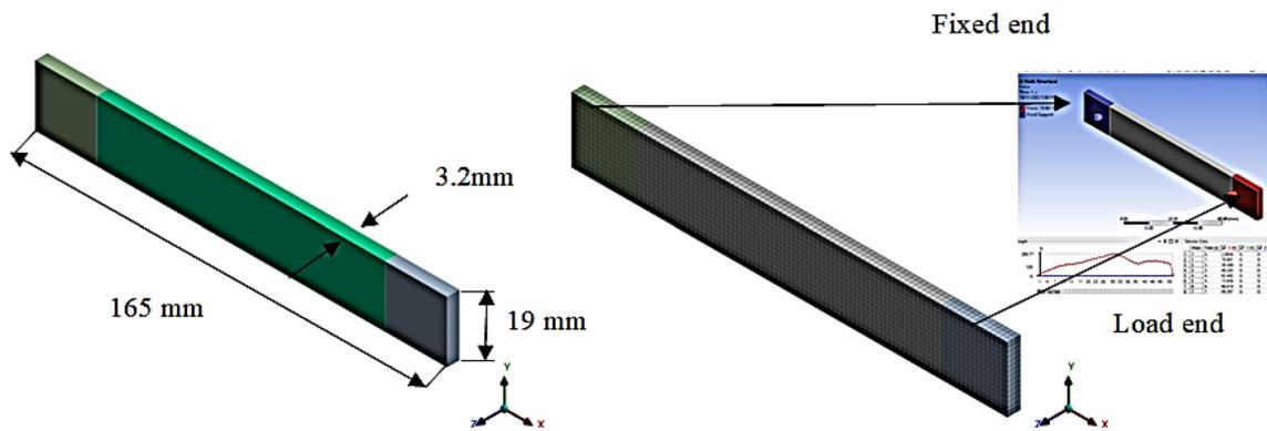
Fig. 8 Geometrical and finite element model of composite with loading and boundary conditions
