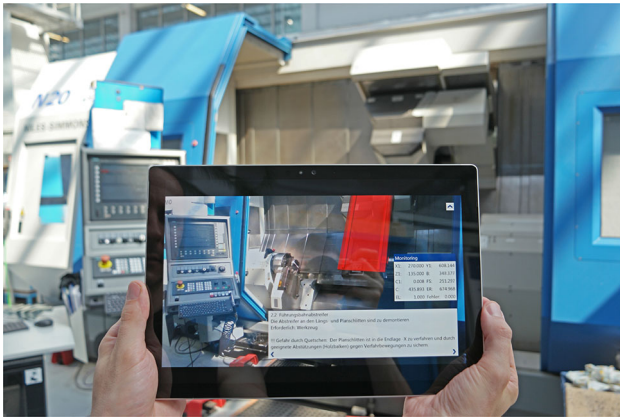
Fig. 10 AR application with the created maintenance documentation
