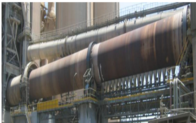
Fig. 1 A typical rotary kiln
