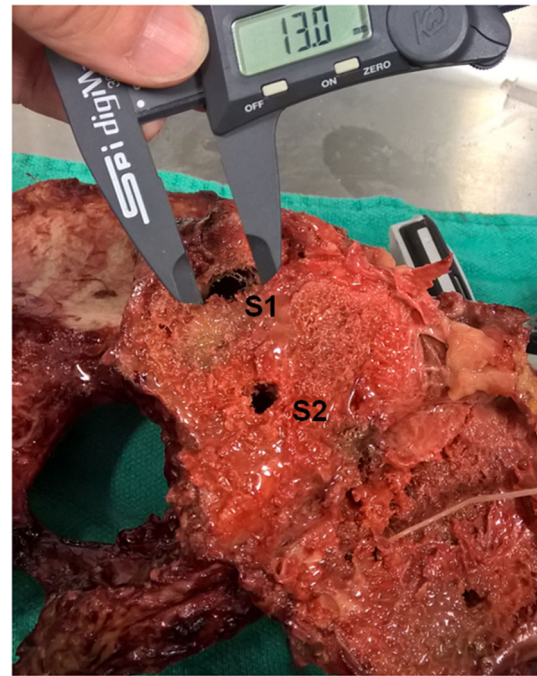
Fig. 5 To determine screw subsidence as an additional measure of screw loosening, the length of the medial-sided screw hole in S1 was quantified from inside the fracture after biomechanical testing. Screw subsidence was defined as the difference between maximum screw hole diameter and the core diameter of the screw.
