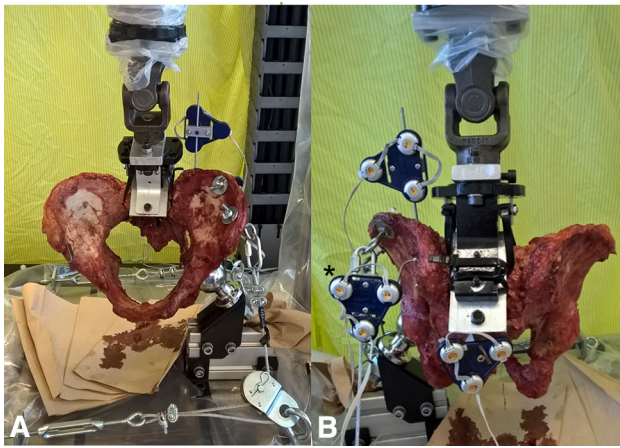
Fig. 3A–B (A) On a universal testing machine, cyclic loadings were applied through the sacrum that was allowed to pivot in all planes while the left hip socket articulated with a fixed femoral head substitute. Hip abductor muscles were simulated by cable pulleys attached to the iliac crest. (B) Displacement under loading was measured using an optoelectronic camera system. Markers were placed on the iliac crest, the sacrum, and the S1 screw (*).
