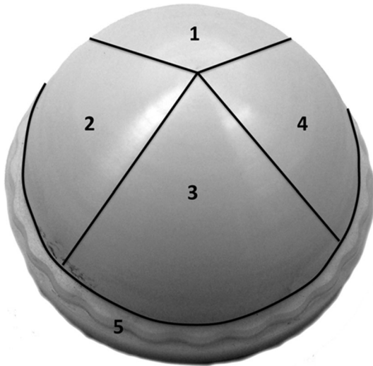
Fig. 2 Grid used for damage scoring has been shown in this image: 1 = anterosuperior; 2 = anteroinferior; 3 = posteroinferior; 4 = posterosuperior; and 5 = peripheral.
