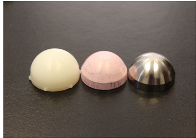
Fig. 4 A taper-lock mechanism may cause the peripheral tabs of a polyethylene liner, unlike the alternate hard bearings, to round over time.
