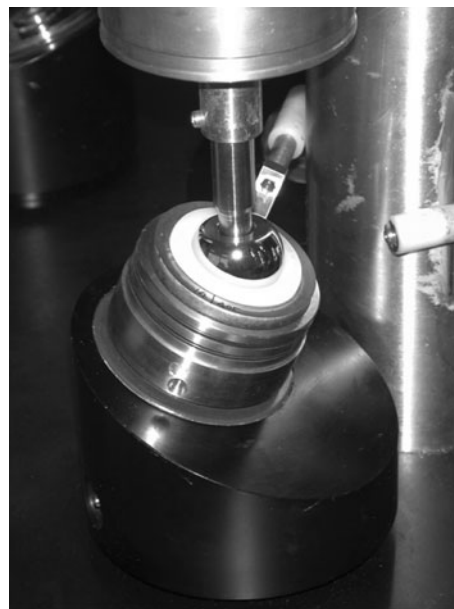
Fig. 3 Details of one test station on the orbital-bearing-type hip simulator show a PE liner in a urethane mold, with the femoral ball loaded from above. During the wear test, an acrylic cylinder encloses the liner to contain the serum lubricant.
