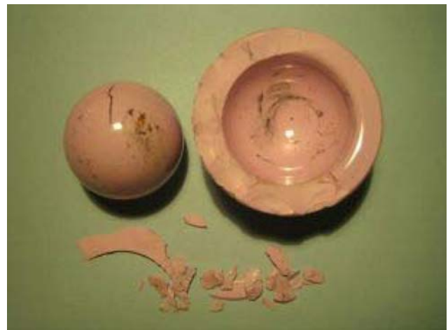
Fig. 3 The retrieved liner and head show the fractured rim of the liner and ceramic fragments retrieved from the wound.
