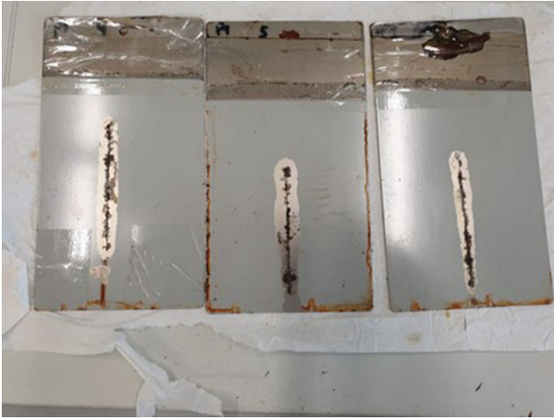
Fig. 70: Sample 6 after 650 h SST. Delamination: \varnothing = 5.3 mm, Corrosion: \varnothing = 0.3 mm
