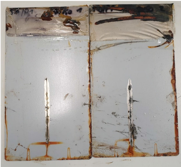
Fig. 74: Sample 2 + sample 6. Delamination: \varnothing = 2.2 mm, Corrosion: \varnothing = 0.3 mm
