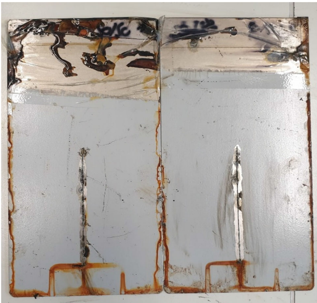
Fig. 75: Sample 2 + sample 7. Delamination: \varnothing = 2.1 mm, Corrosion: \varnothing = 0.3 mm
