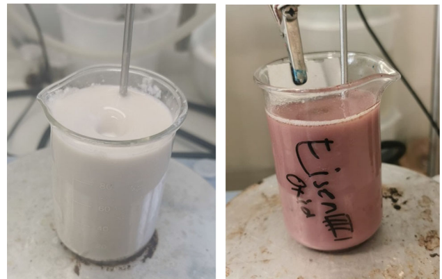
Fig. 77: The dip bath from sample 1 (left) and sample 1 with 0.05 g iron oxide (right)
