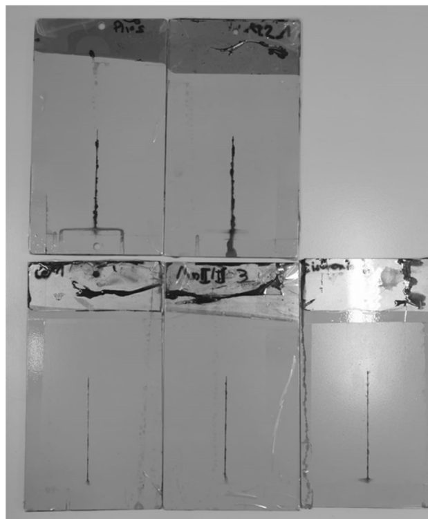
Fig. 31: Sample 1 with different oxides after 500 h SST in the following order from the top left to the bottom right [phosphated steel, Sample 1, Ce(IV), Mn(II/III), iron oxide]
