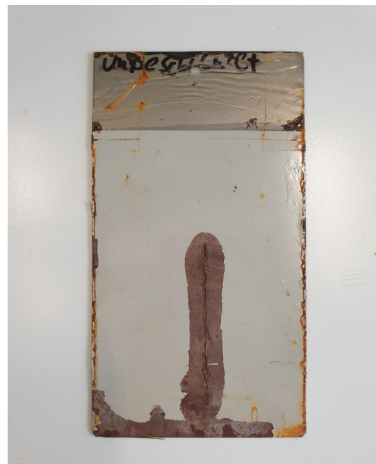
Fig. 69: Noncoated steel after 650 h SST. Delamination: 8.9 mm, Corrosion: 0.1 mm
