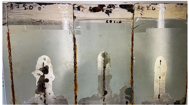
Fig. 73: Sample 2 after 650 h SST. Delamination: \varnothing = 12.2 mm, Corrosion: \varnothing = 0.5 mm
