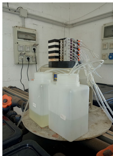
Fig. 4: Experimental setup for the obtainment of the pH and free chlorine, free-Cl, conditions presented in Fig. 3: (a) general scheme; (b) picture of the peristaltic pump for the addition of NaClO and HCl 1 M solution
