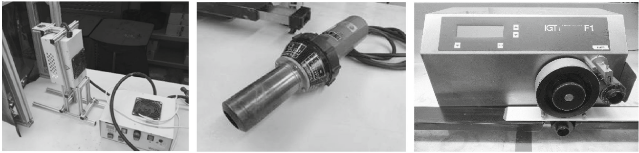
Fig. 2: Set-up for UV-curing (left), hot air blower (middle), and laboratory flexo printing machine IGT F1 (right) used in the experiment
