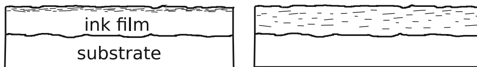
Fig. 1: Distribution of leafing (left) and non-leafing (right) aluminum pigments in ink. In the left, pigments float up to the ink film surface after printing. In the right, they stay evenly distributed in the ink. In this study, using VMPs in UV-inks, we are faced with the left situation
