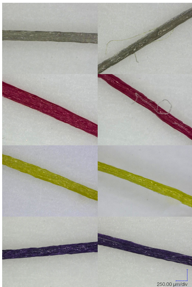
Fig. 8: Micrographs of PA multifilament yarn after coating (left) and after Martindale abrasion test (right) filament yarn after coating
