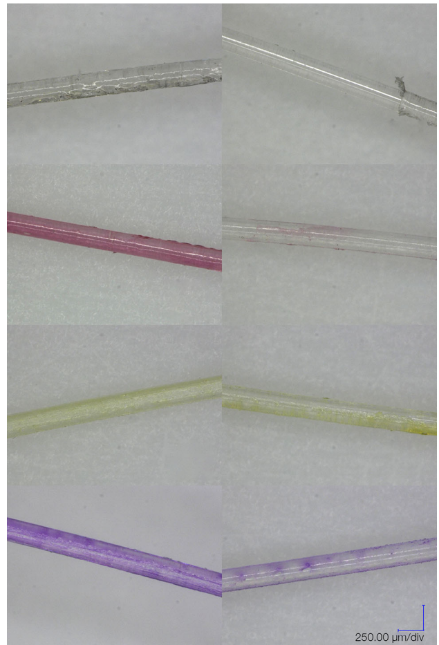
Fig. 7: Micrographs of PET monofilament yarn after coating (left) and after Martindale abrasion test (right). Colors are according to table (Color figure online)
