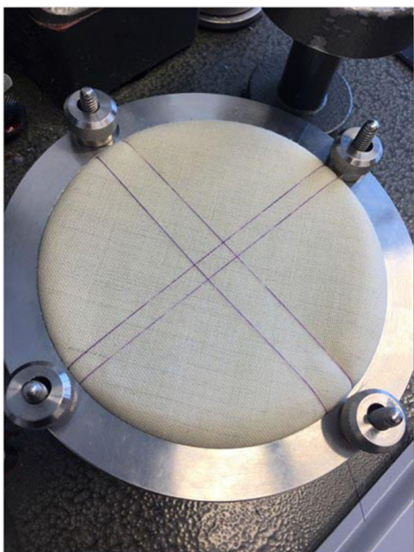
Fig. 3: Modified Martindale abrasion test for r-PVB-coated yarns
