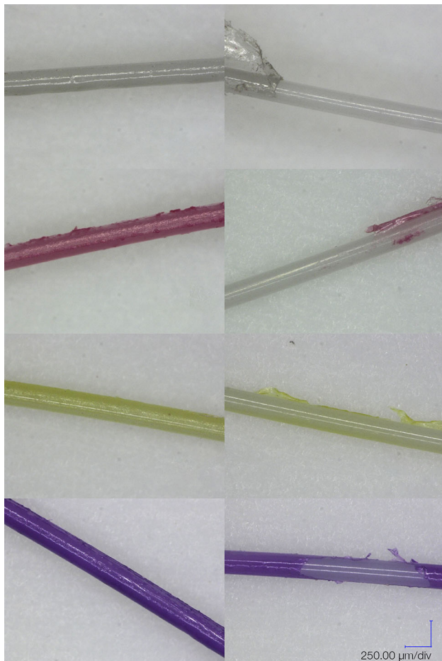
Fig. 6: Micrographs of PA monofilament yarn after coating (left) and after Martindale abrasion test (right). Colors are according to table (Color figure online)
