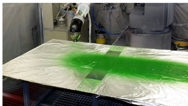
Fig. 6: Measurement setup to determine film thickness distribution—dynamic spray pattern
