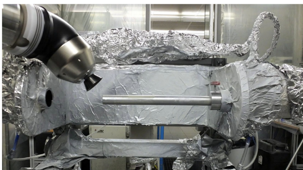
Fig. 5: Measurement setup to determine particle size distribution by means of laser diffraction
