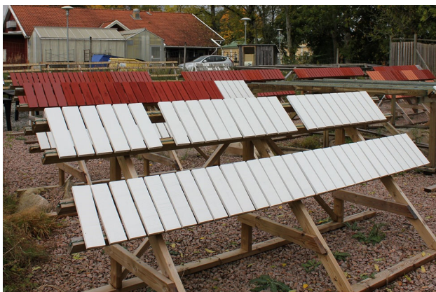
Fig. 2: Exposure racks for samples at test field
