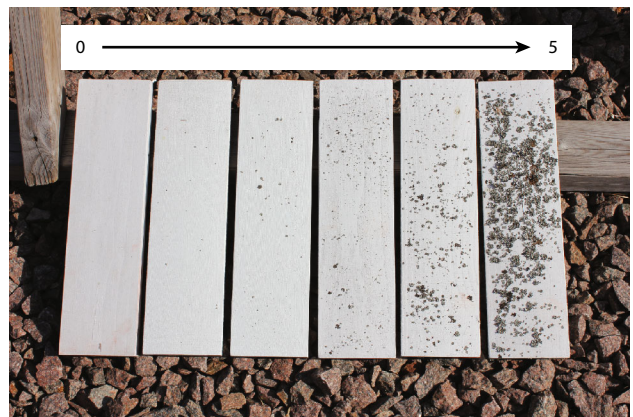
Fig. 3: Grading scale of biological growth. Grade 0 = no detectable defects/biological growth. Grade 5 = dense pattern of defects/biological growth
