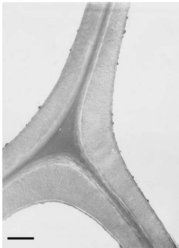
Fig. 6: Low magnification TEM micrograph showing typical appearance of untreated tracheid walls of untreated P. radiata in terms of staining characteristics of various cell wall regions. \text{KMnO}_4 staining. Bar = 2 \mu\text{m}
