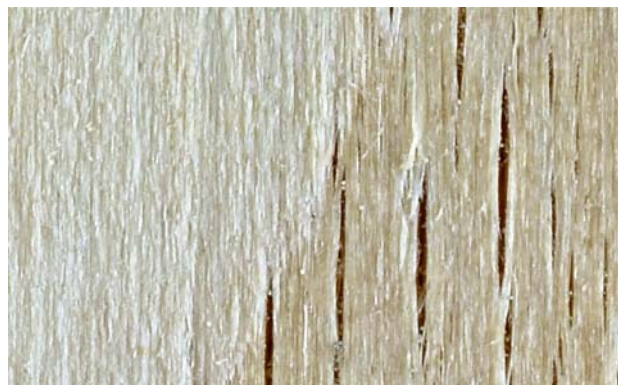
Fig. 3: Latewood more heavily checked than earlywood following peracetic acid treatment
