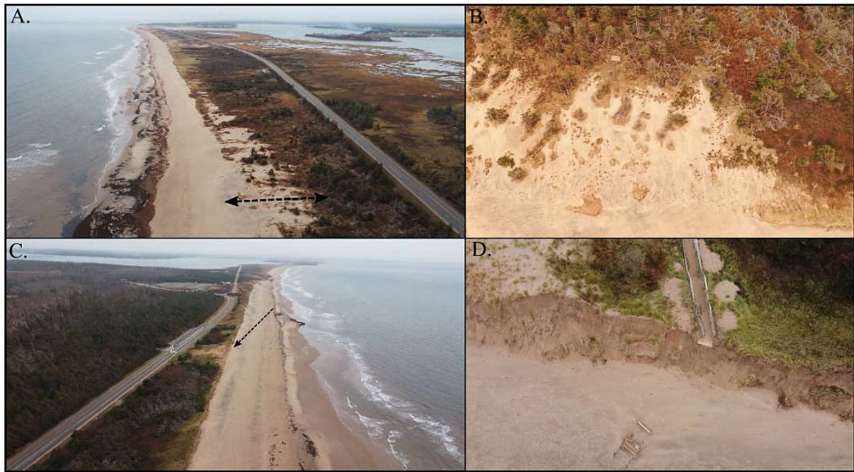
Fig. 15 Overwash penetration and crest retreat at Brackley Beach following the impacts of Fiona. Photograph A was taken above Brackley Main Beach, the arrow delineates approximately 30–40 m of overwash deposition, further depicted in image B. Image C was taken above Shaw’s Beach to the east of Brackley Main, facing west towards
