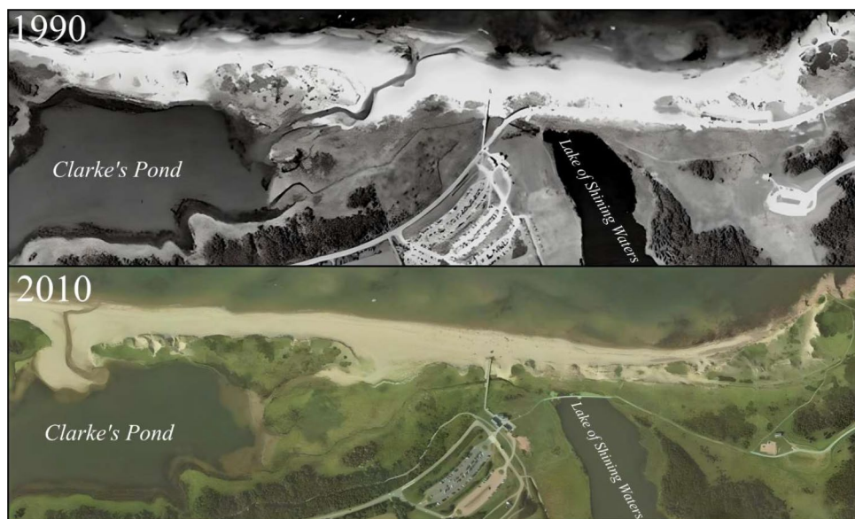
Fig. 5 Cavendish Main Beach historical imagery, east of the spit and campground. By 1990, removal of a parking lot east of the boardwalk allowed vegetation to re-establish in this area and along the main foredune. By 2010 pressure on the foredune was reduced by removing the roadway across the lee of the foredune slope and replacing it with a trail and boardwalk across the Lake of Shining Waters
