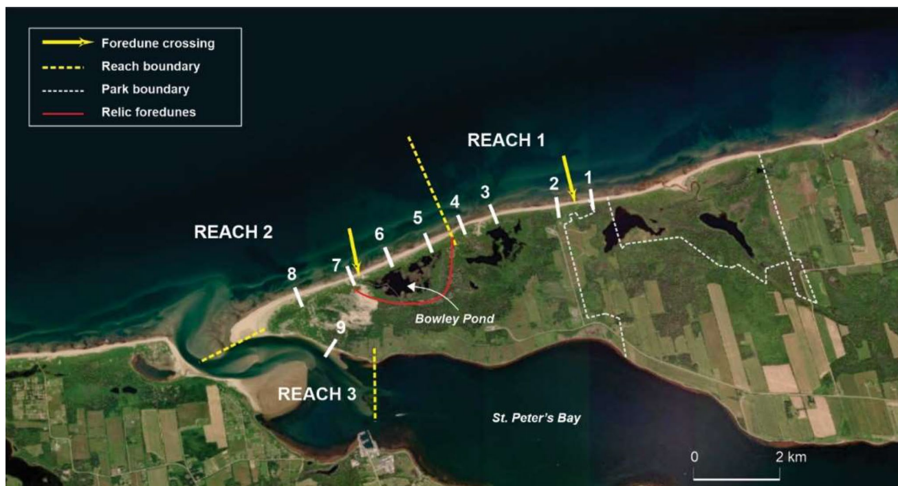
Fig. 2 Satellite image showing the shoreline at Greenwich. The locations of the 9 Lines across the beach and foredune which were monitored from 2002–2023 are shown together with the three reach boundaries and the location of the two dune crossings on the exposed beach
