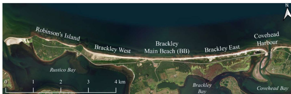
Fig. 6 Satellite image of Brackley Beach from Robinson's Island in the west to Covehead Harbour at the eastern end. The section of foredunes west of Brackley Main Beach (BB) are characterized by a large washover channel and prograding dunes of low crest elevation. BB contains a continuous foredune system \sim 4 m in height, and has the
