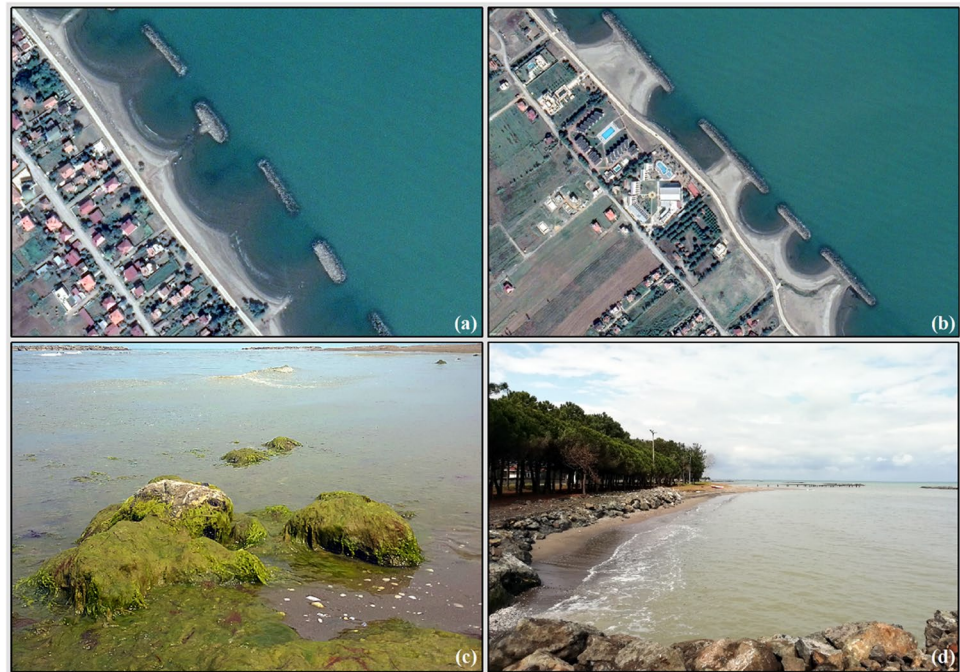
Fig. 9 Environmental impacts of coastal protection structures. a Filling areas formed by the accumulation of sand between the groins (GE Pro 7.3.4.8642, September 17, 2019). b Tombolo-like formations resulting from the merging of offshore breakwaters with the coast (GE Pro 7.3.4.8642, September 17, 2019). c Presence of algae and pollution between coastal protection structures (June 11, 2020). d Coastal fortification with rock/stone fill laid along the seaside (March 27, 2021)
