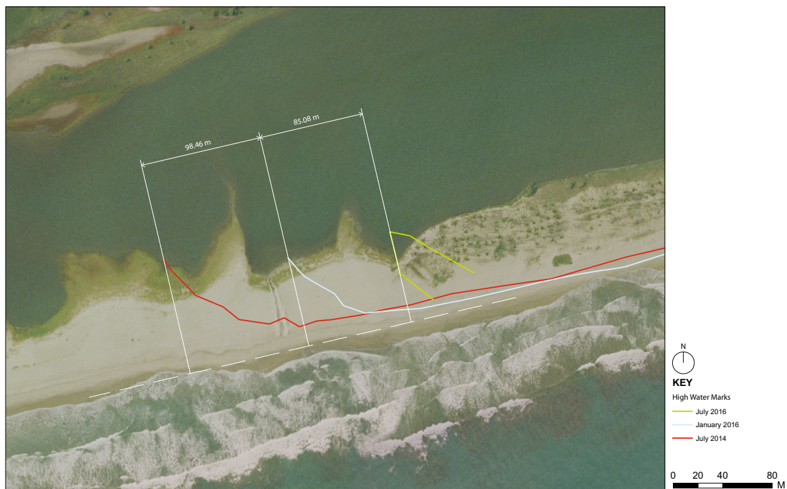
Fig. 4 Positions of the eastern (barrier) side of the breach in July 2014, January 2016 and July 2016 plotted onto 2005 aerial image
