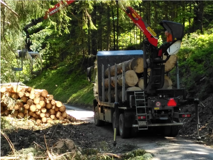
Fig. 4 Piling of assortments by truck
