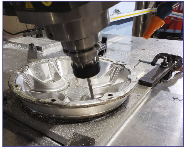
Early stages of manufacturing a cryogenic tank with integral cooling passages.
