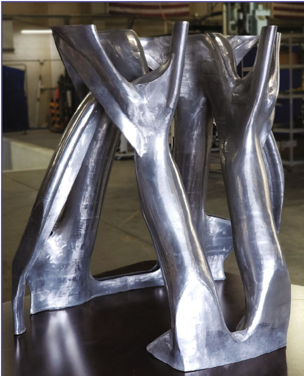
This optimized lightweight airframe structure has interior and exterior machined surfaces. Photos provided by Big Metal Additive.
