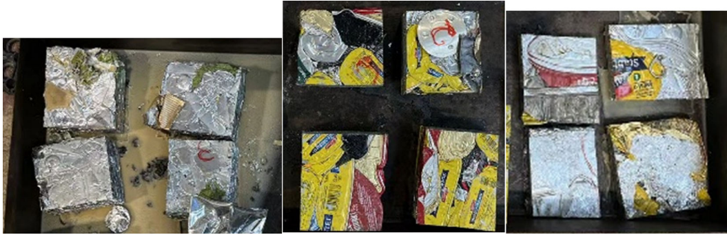
Fig. 4. Al fraction in the supermarket pilot after 24 h thermal treatment in air at 110°C: laminated and dirty scrap (left), clean and coated scrap (middle), and clean and without coating scrap (right).
