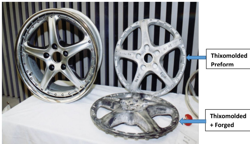
Fig. 7. Auto wheel Thixomolded and forged by Mazda and Japan Steel Works.
