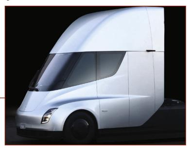
Palo Alto, California, USA: Tesla entered the semi market with the launch of its heavy-duty all-electric truck. Highlighted at the launch event in November 2017 were the vehicle's range of up to 500 miles, energy consumption of less than 2 kWh/mile, and the ability to accelerate from zero to 60 mph in 20 seconds. (Image, right, courtesy Tesla Motors.)
