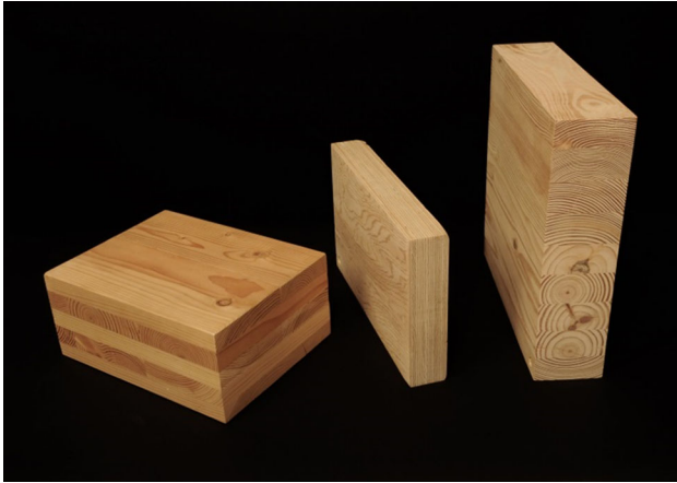
Fig. 3. Massive timber composites. From left to right: cross-laminated timber (CLT), structural composite lumber (LVL), and glulam.
