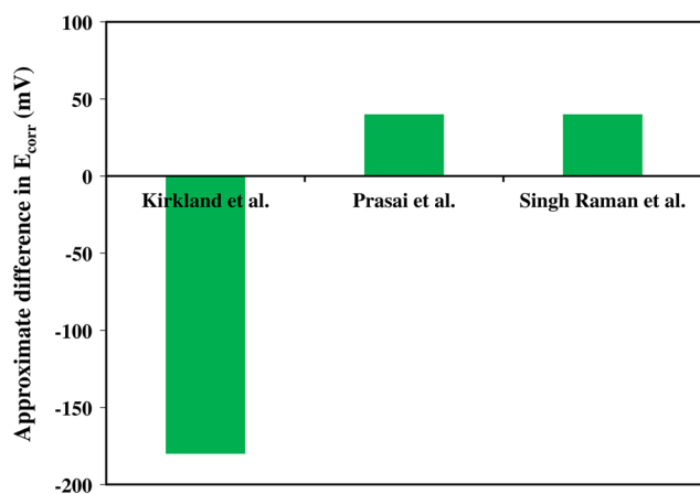
Fig. 4. Difference in the E_{\text{corr}} of the graphene-coated and uncoated Cu as reported in the studies by Kirkland et al., 7 Prasai et al., 5 and Singh Raman et al. 8 (Reprinted with permission from Ref. 1, Copyright 2012 Australasian Corrosion Association Inc.)
