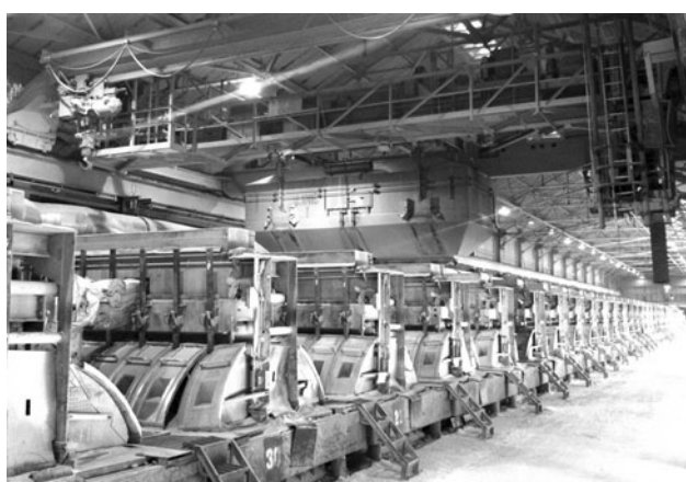
Fig. 5. Filling of alumina bins on pots from a crane-mounted bucket (provided courtesy of Alcoa, Inc.).
