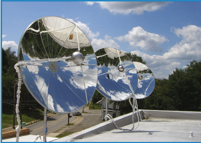
Inexpensive, 8-foot stamped steel satellite dishes make Epiphany's parabolic concentrator array easy to acquire, set up, and maintain in the remotest corners of the world. (Photo courtesy of Epiphany Solar Water Systems.)
